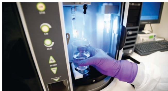
**Solution collected from a simulated-use model is placed in a particle detection system to count and size the particulate generated.**
