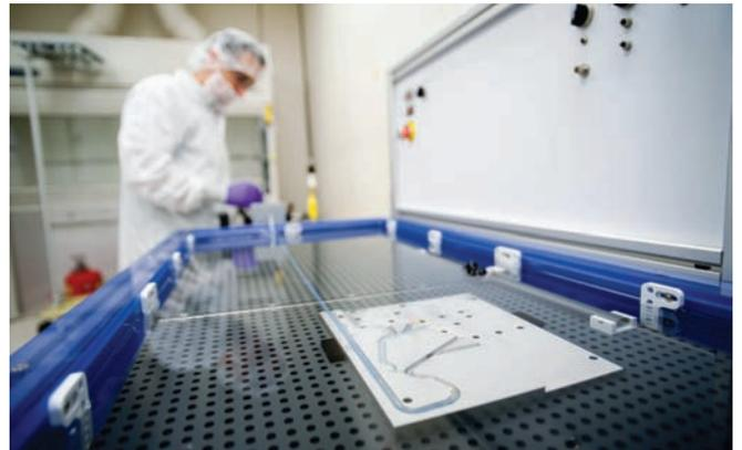
**A coronary simulated-use model is used to evaluate both friction and particulate properties of a PTCA catheter.**
